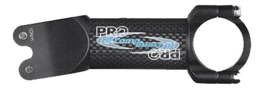
PRO has identified a potential safety issue involving the PRO Hi-Comp road racing bicycle stems produced between November 2003 and June 2006. Due to fatigue these stems may crack and eventually break. If this happens during cycling, the cyclist may lose control of the bicycle, which could lead to serious injuries.
